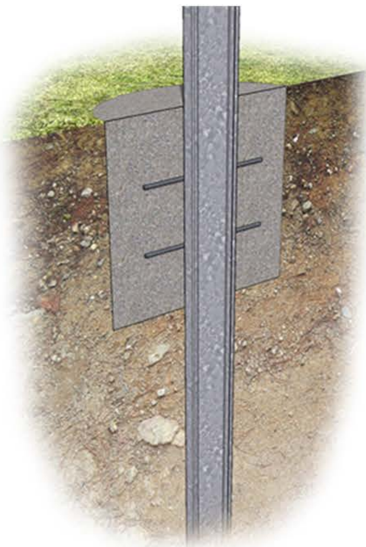
Ramming with concreting
